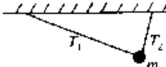
5. A ball of mass  $m$  is suspended from two strings of unequal length as shown above. The tensions  $T_1$  and  $T_2$  in the strings must satisfy which of the following relations?
