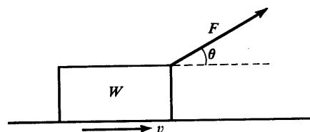
4. A block of weight  $W$  is pulled along a horizontal surface at constant speed  $v$  by a force  $F$ , which acts at an angle of  $\theta$  with the horizontal, as shown above. The normal force exerted on the block by the surface has magnitude
