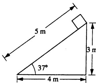
A plane 5 meters in length is inclined at an angle of  $37^\circ$ , as shown above. A block of weight 20 newtons is placed at the top of the plane and allowed to slide down.
